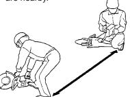
Figure 1. Start the engine at least 3 meters from a fueling location.
